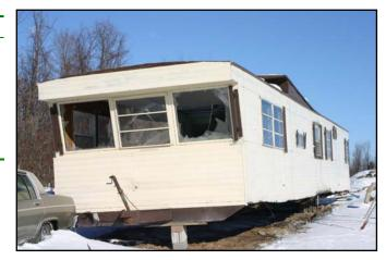
**Exterior:** The siding is metal, and there is a lot of large junk items and debris around the trailer, including an old car parked close by. It was lifted on cinder blocks at the near end in the above photograph, and supported on axle and wheels at the far end. Many of the
